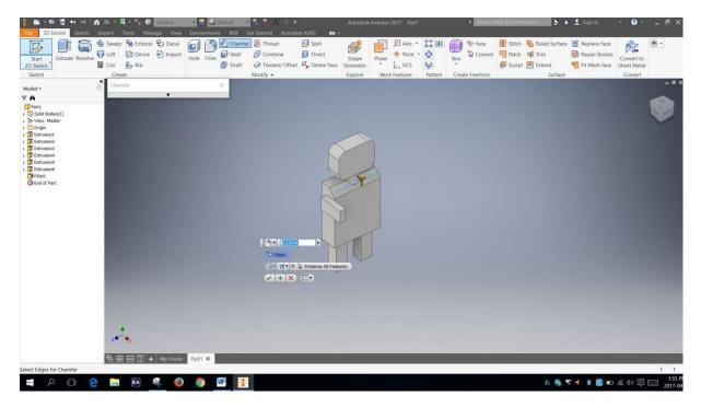
Step 10: If prefer to chamfer your edges, select the Chamfer tool in the navigation menu and select the edges you want to chamfer. Click the green check mark when you are done.
