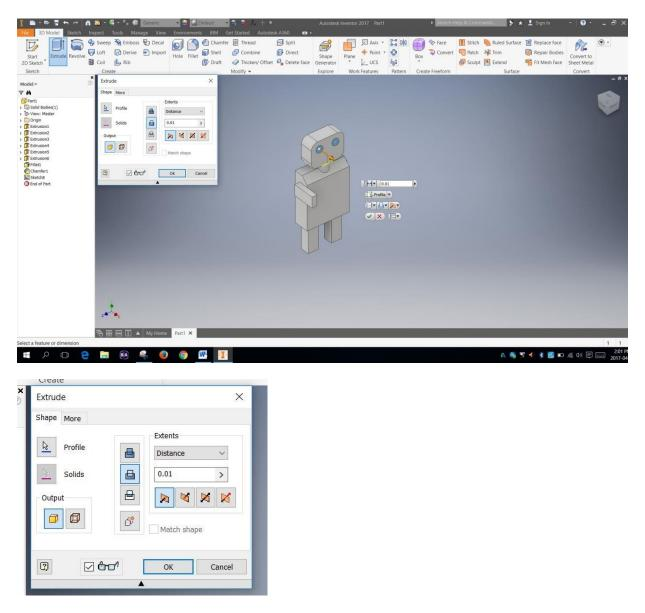
Step 11: To cut a shape you have drawn into the face as opposed to extruding the shape out of the face, select Extrude and then the Cut function in the Extrude menu. Adjust the depth of the cut by modifying the distance in the number box in the menu. Select the OK tab or the green checkmark when you are finished.
