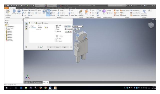
Step 9: After you have extruded the shape of the features, if you wish, you can use the Filet function to produce curves instead of the sharp corners. After selecting the Filet tool in the navigation tab, select the edges you wish to filet and enter the magnitude of filet of your choice in the number box. Click the green checkmark when you're finished.
