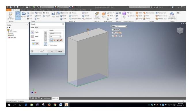
Step 6: To make your shape drawn into a prism; select the Extrude tool on the navigation menu.
