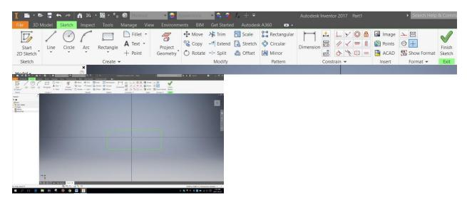
Step 4: After you selected your plane, the sketch tab shown above should be activated. Select the tool (rectangle, circle, line or arc tool) and begin sketching your shape. You can edit the dimension of each of your lines by selecting Dimensions and then selecting your line. Enter your preferred dimension into the number box. Please note that your sketch must be a closed shape. Double check if all your lines meet.
