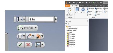
Step 7: Enter the height you want your object to be in the number box and select the green checkmark when you are finished editing. You can always edit the Extrusions you have made by double clicking the Extrusion displayed on the menu on the left of the working window.
